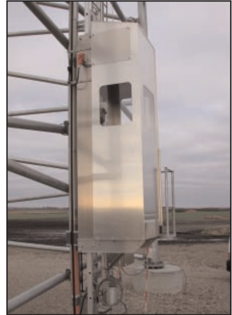
Pro-Bel TH250-U Tower Hoist Personnel Cage used in exterior application. Note cover on top to protect electrical components and power conductor rail instead of trailing supply cable.
